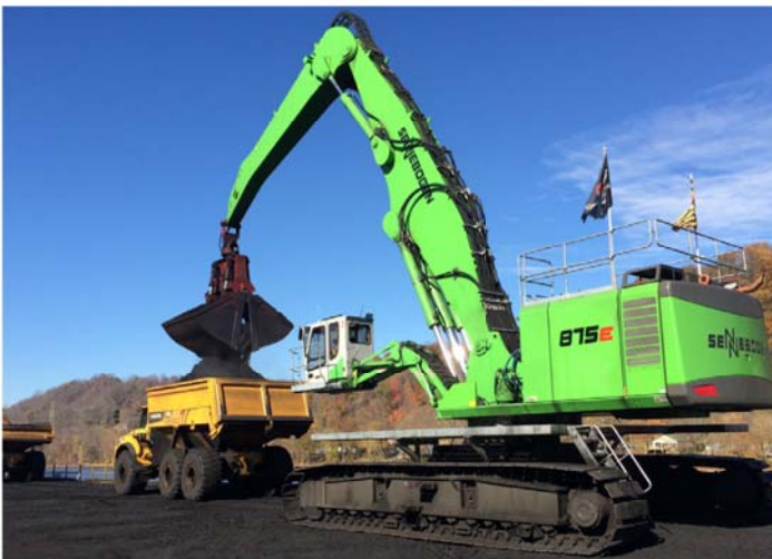
Coal handling using a double-shell grab, USA
