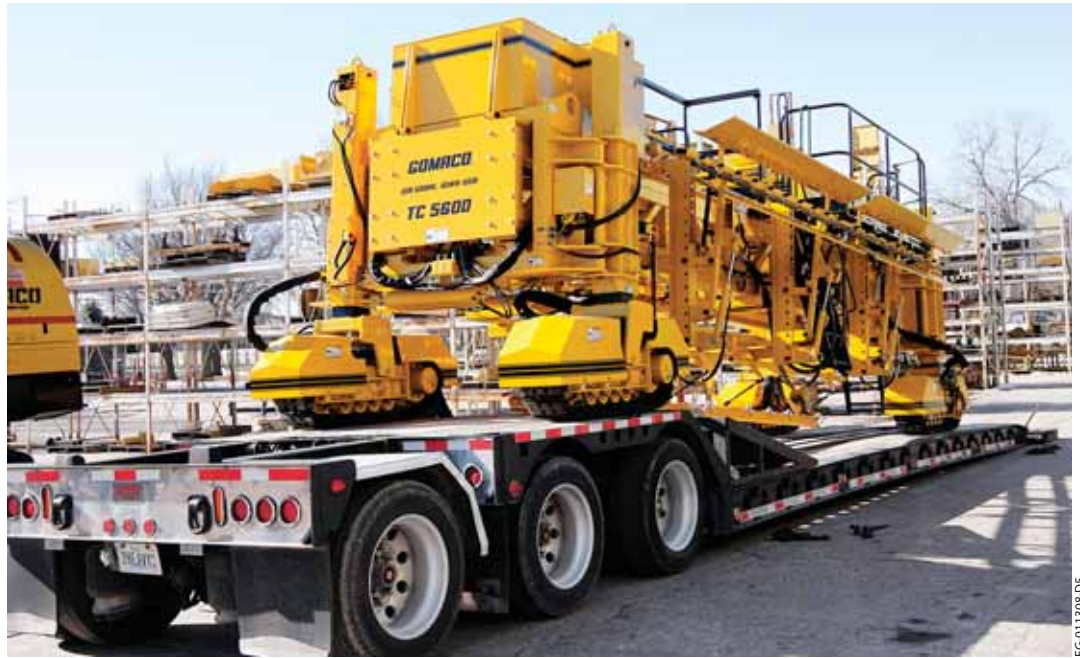
The four-track T/C-5600 texture/cure machine can turn its tracks 90 degrees to drive onto a trailer for transport.
