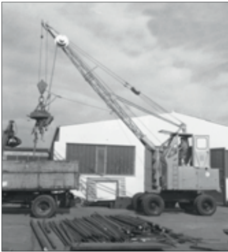
1962: rope-driven S833 with elevated operator cab
