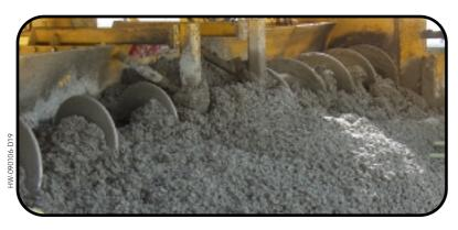
The spreading of either concrete or base material is quick and accurate with the reversible 20 in. (508 mm) diameter hydraulically powered split auger. The hydraulically pressure-compensated sideplates provide edge control and a spreading depth up to 19 in. (483 mm).
