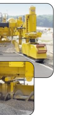
PS-4000 conveyor is designed extends in seven seconds and conveyor deflector directs the crial for the paving operation.
