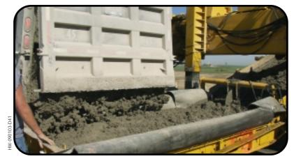
The GOMACO-designed conveyor system on the PS-4000 provides quick, clean and efficient delivery of concrete to the grade.
