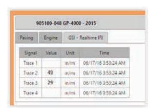
One option for viewing the GOMACO GSI smoothness data in real-time with the GRD software is to see it in table format.
