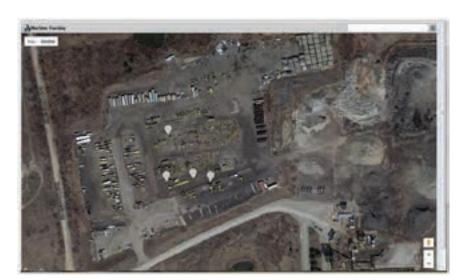
The white dots on the above map show the exact location of the GOMACO machines by mapping them through GPS positioning. This screenshot example shows all of the company's GOMACO machines are located within the company's storage lot.
