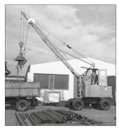
1962: Rope-driven S833 with elevated operator cab
