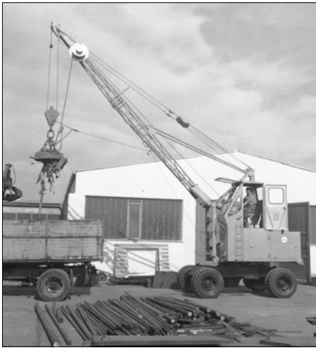
1962: rope-driven S833 with elevated operator cab
