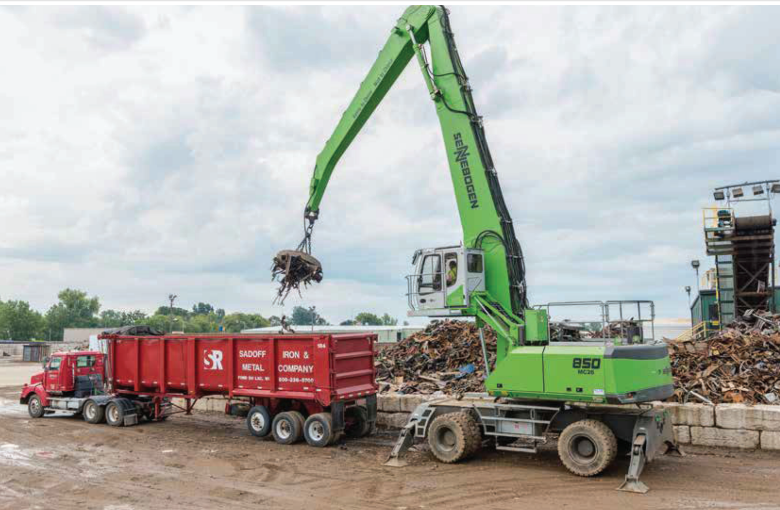
26 850 M - with magnet plate - truck loading; USA
