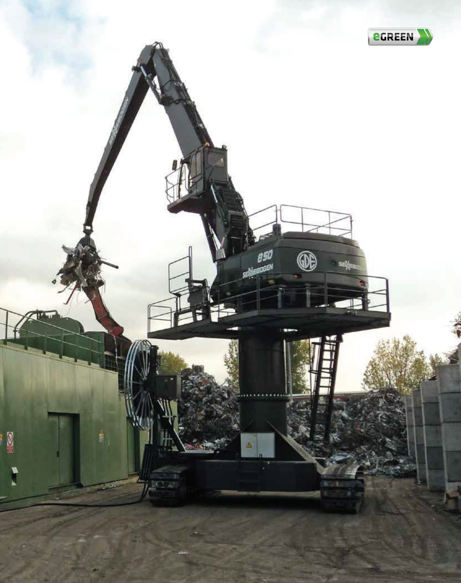
850 R special electro - with orange peel grab - loading of a scrap shear; France
