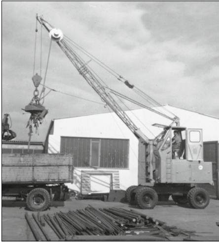
1962: Rope-driven S833 with elevated operator cab
